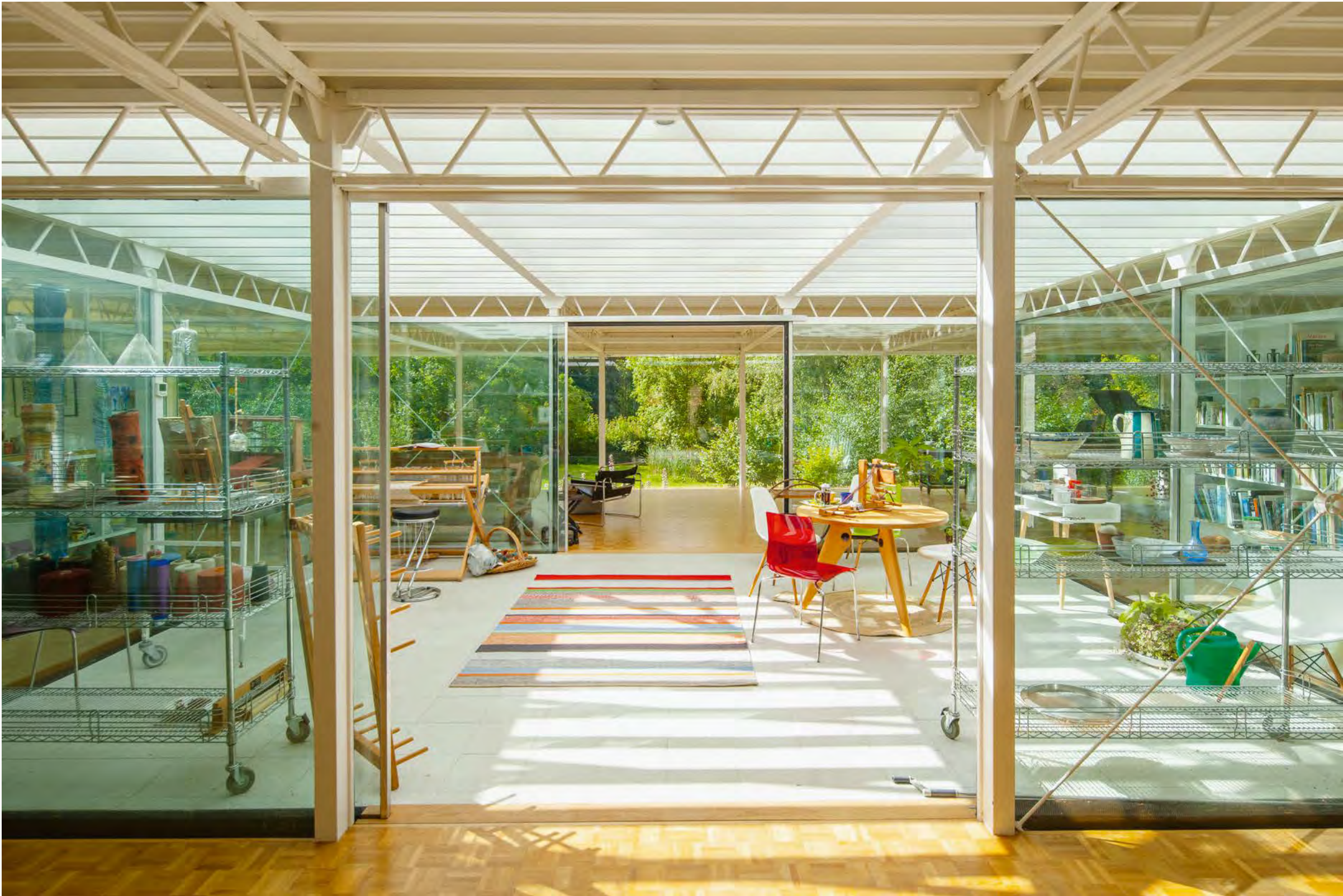
Right: the same sized steel lattice trusses are used for the perimeter and exposed internal structure throughout the house, attached to a regular grid of slender steel columns
